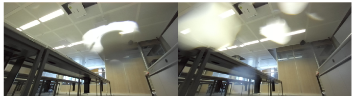
FIGURE 4.5: Stereo Image taken in RVIZ with sprayed lens
