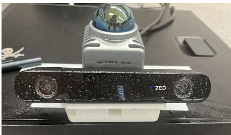
FIGURE 4.4: Camera after being sprayed with water
